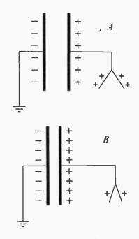
Fig. 1. Principle of the capacitance micrometer.
