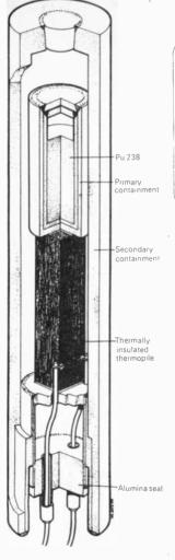
Fig. 9. Isotope battery developed for experimental heart pacemaker. Approximate size is 1.75" x 0.7".
