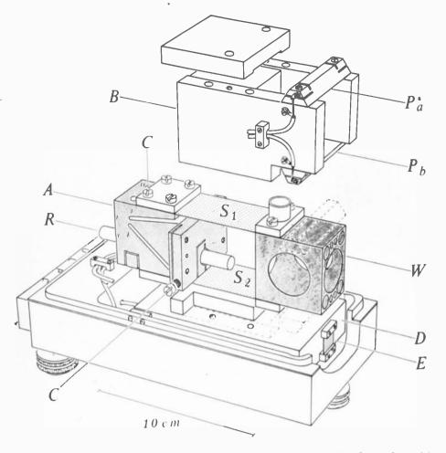
Fig. 2. Gravimeter, in which suspended weight W is held by cantilever springs S<sub>1</sub> and S<sub>2</sub>, which deflect vertically by about 5mm because of the gravitational pull on W. Small changes in the position of W, due to changes in 'g' are recorded by the disturbance of the bridge formed by W, P<sub>P</sub>, and P<sub>D</sub>.
