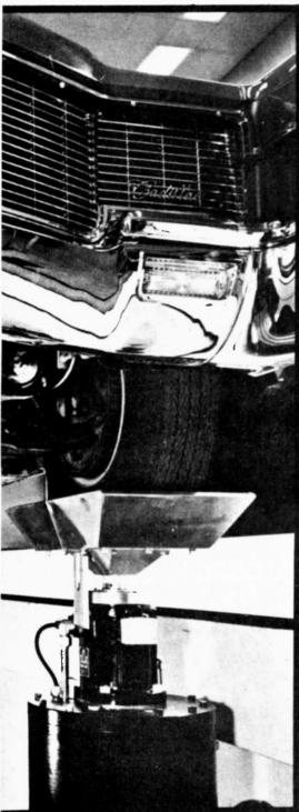
Detail view of electro-hydraulic actuator, hydraulically operated floor is raised when car is driven onto the simulator, then lowered to allow access to all parts of the car during test.
