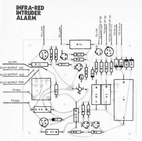
Fig. 4. How the components are located on the printed circuit board.
