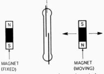
Fig. 3. A fixed megnet of opposite polerity to the moving megnet may be used to reduce pull-in, pull-out differentiel.
