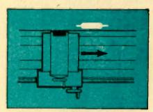
Position control and indication, obviating mechanical contact with its implications of wear, and simplifying mounting.
