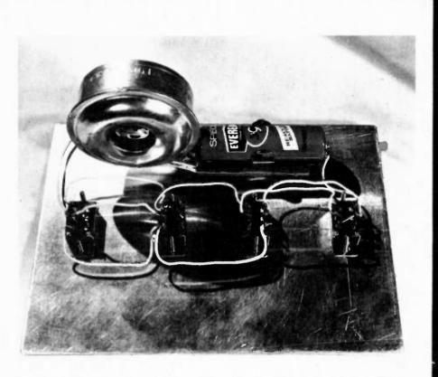
Fig. 3. How the unit is constructed - compare this with the wiring diagram shown in Fig. 4.
