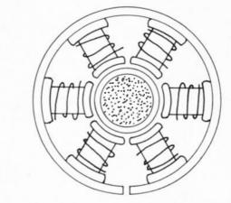
Fig. 1. A ring of coils can produce a rotating magnetic field.
