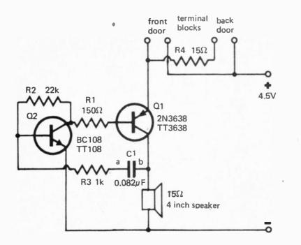
ERE is a simple door monitor that produces a different tone for either of two buttons connected to it.
