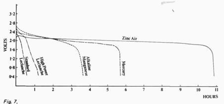
Discharge curves of various types of cell compared to a zinc-air battery of the same physical size.
