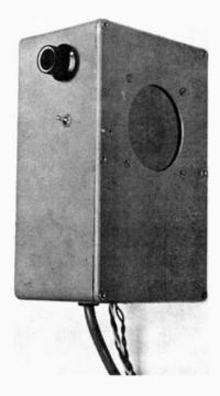
because they are readily obtainable, easy to drill and cut, and when finished result in a really professional product. An alternative construction might well employ timber boxes made out of marine quality plywood.
