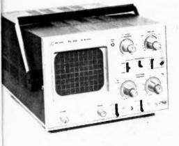
Extensive use of "automation in operation" facilities and full overload protection of inputs are important features of an easy-to-use 50 mV/cm dual-trace oscilloscope just introduced by Philips.
