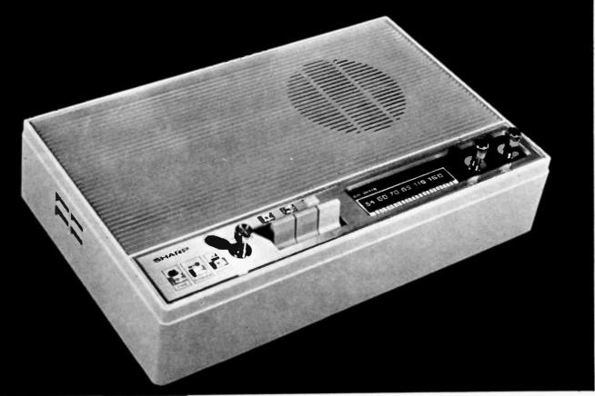
The Sharp Home Keeper is a concentrated control system equipped for interphones, fire detector, buzzer, pool alarm, theft alarm switches and radio set. Various equipment can be connected to this device in order to assure safety in your house. In the package is the main consul, doorphone, five theft alarm switches, three fire detectors, pool alarm and overflow, temperature and leak detector and intercom for babies room, den or bedroom. Extra fire and pool alarm units are available as required.
