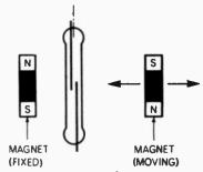
Fig. 4. 'Normally closed' operation can be obtained by biasing a 'normally open' read switch with a fixed magnet. The moving magnet cancels out the fixed magnet and thus allows the switch to open,
