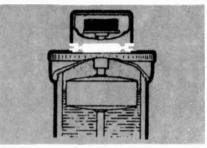
Hydraulic brake fluid level indicator, where feasibility depends on simplicity and ease of application.
