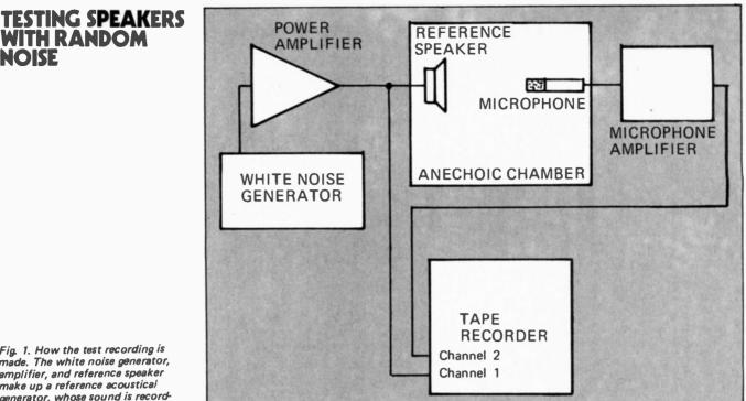
Fig. 1. How the test recording is made. The white noise generator, amplifier, and reference speaker make up a reference acoustical generator, whose sound is recorded in an anechoice chamber.
