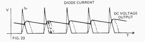
This is the peak current which the diode will conduct on each fluctuation, The diode peak current rating must, therefore, be in excess of the value which is calculated from the above.
