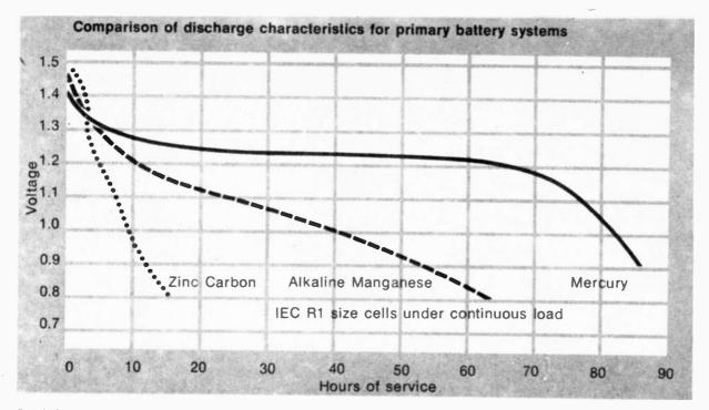
Fig. 4. Graph shows discharge performance of zinc-carbon, alkaline manganese and mercury batteries.
