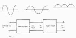
This provides an almost steady dc, there remaining only the problem of being sure that the supply maintains a steady flow of power and does not allow fluctuations. For this, a control circuit is added to counteract fluctuations in supply or load.
