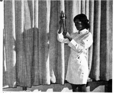
Scientist uses Negretti and Zambra hygrometer whilst testing characteristics of curtain material.
