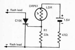
In photography, a separate flash, triggered by the light of a master flash light, is often required to provide more light, fill-in shadows etc.
