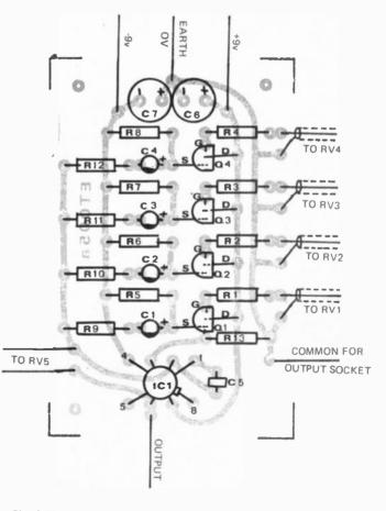
Fig. 4. How components are mounted on the printed circuit board seen from components side.
