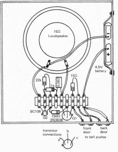
Fig. 2. Wiring diagram showing component layout.
