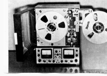
The concentrically mounted tape reels swing apart for easy tape loading.
