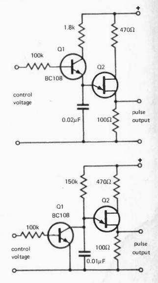
Voltage controlled pulse oscillators find a wide variety of applications in telemetry, SCR control systems, analogue to digital converters etc.
