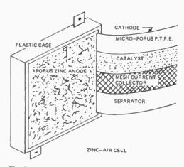
Fig. 6. Section of rectangular zinc-air cell.
