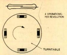
Fig. 8. Simple yet versatile impulse timer can be improvised by placing one or more magnets on a gramaphone turntable.
