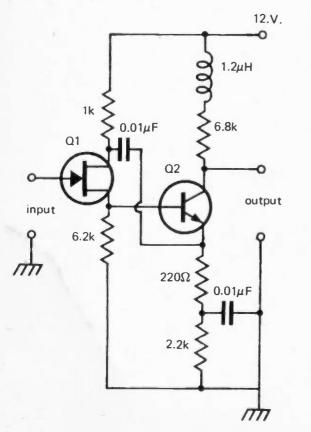
This circuit has a typical gain of 10db and bandwidth of 90 MHz.
