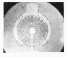
A new series of transistors from Hewlett Packard combine good power output and gain, in the gigahertz region.
