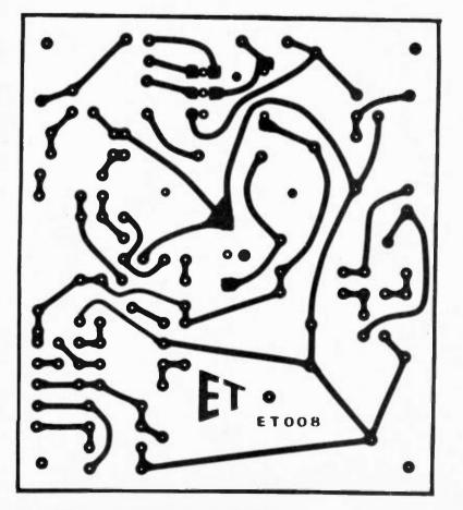
Fig. 5. Foil pattern for printed circuit board - full size.
