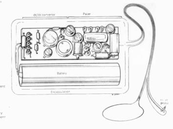
Fig. 10. Drawing of complete isotope powered pacemaker.
