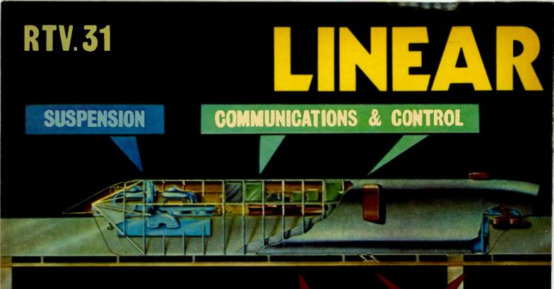
The experimental tracked air cushion vehicle, which Tracked Hovercraft Limited aims to have under full-scale test this year is shown cut-away to indicate the amidships positioning of the 6,500 lb thrust single-sided linear motor used for propulsion, and the hoverpads used for support and guidance. The vehicle is designed to reach 300 mph, towards the end of 1972, when the test track at Earith, in England is extended to eight miles in length.
