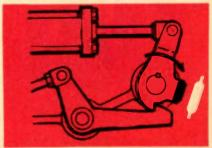
Safety interlock switching, giving extreme reliability and simplicity of application to complex mechanical layouts. Reed insert completes circuit to illuminate warning lamp or permit further stage of operation.
