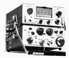
Among the features of the 1401A-1 Spectrum Analyzer is automatic center frequency positioning in a "search" mode. At 50 MHz/div frequency span (dispersion), the center frequency automatically becomes 250 MHz, preventing an erroneous display. In "search", the center frequency control positions a negative marker to indicate that part of the spectrum which will appear at center screen when the frequency span is reduced to less than 50 MHz/div.
